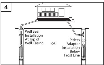
4a. Pitless Adaptor Installation. Pitless adaptor should be installed below the frost line, and on the side of the well casing where the supply line will run from well, in accordance with the manufacturer's instructions. (Fig. 4a)
