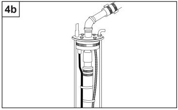
**WARNING:** All electrical wiring or service should be done by qualified electrician. Be sure to test cable for continuity with an ohmmeter before starting the pump.
