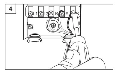
Connect the green ground wire from the pump to the green ground screw in the lower right corner of the control box.
