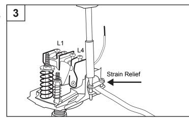
4. Connect the two wires from the house electrical service to the outside pressure switch terminals (L1 and L4). (**Fig. 4**)
