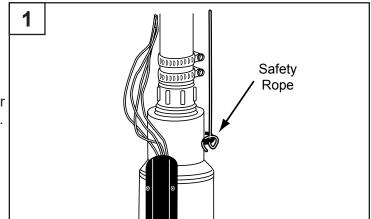
**CAUTION:** Be sure the top edge of the well casing is perfectly smooth. Sharp or jagged edges can cut or scrape the cable and cause a short. Do not let the cable drag over the edge of the well casing since this may cause damage to the insulation.
